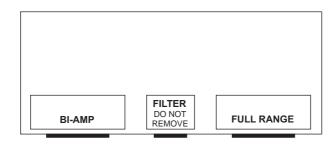
To select the operational mode it is necessary to open the connection panel. Remove the internal connector from the FULL RANGE position to BI-AMP and vice-versa. Do not move, for any reason, the central FILTER connection.
